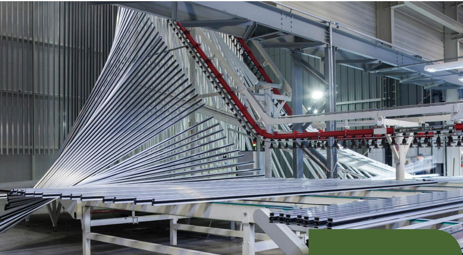
**Above** – The conveyor is feeding in to one of our two vertical powder coat paint lines..
