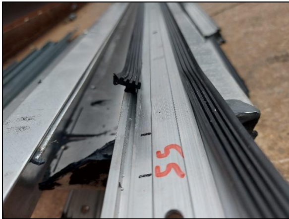
Photograph No. 13 - Pressure plate gasket profile
