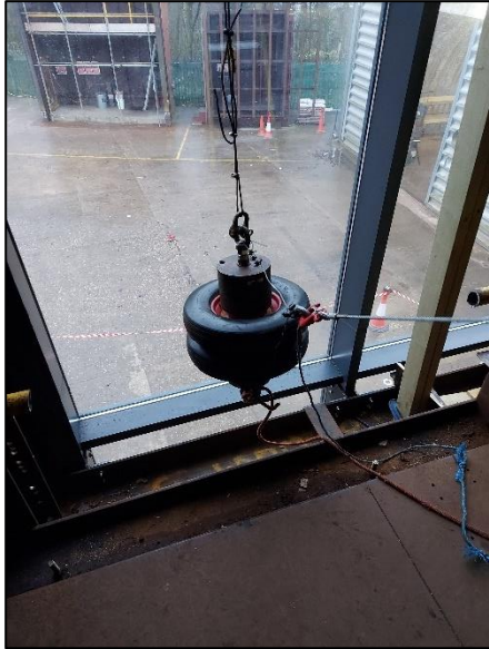
Photograph No. 4 - Showing impactor during internal testing
