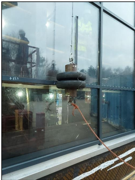
Photograph No. 6 - Showing impactor during external testing
