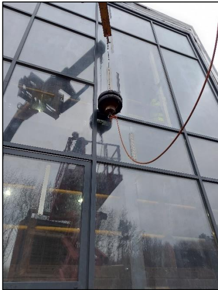
Photograph No. 5 - Showing impactor during external testing
