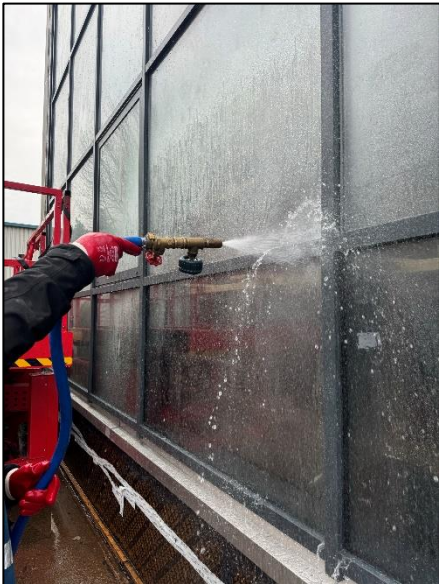
Photograph No. 2 - Hose Test
