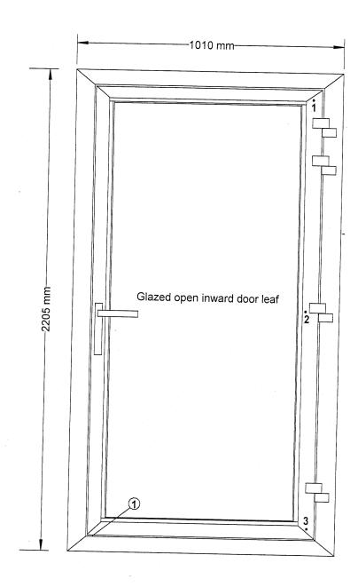
Figure 1. Outline sketch of the inside face of the door showing positions of deflection measurement points on the right hand door leaf stile and point where water leaked through the door at 450 Pa
