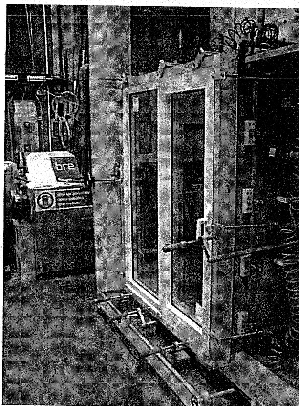
Figure 1. The Smart Systems Eco Futural window with tilt and turn opening light and fixed light in the BRE Test rig 'G'
