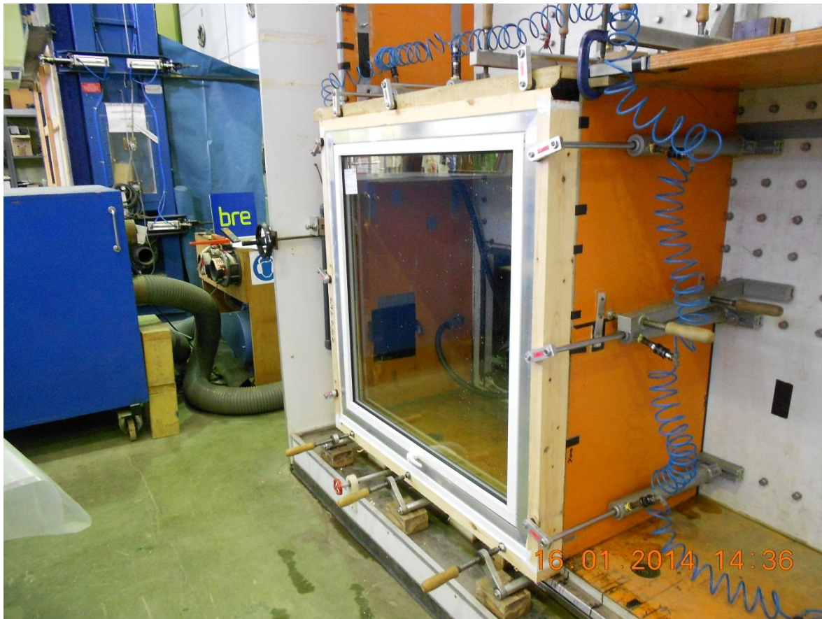
Figure A2. The test specimen mounted in BRE Test rig 'G'
