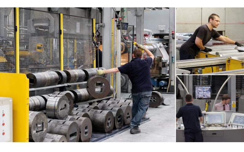
All of our extrusion presses use the latest manufacturing software to minimise production waste – whilst maximising the efficient use of aluminium billets. 100% of the waste aluminium from the extrusion process is captured and then recycled into aluminium billets for future production and as a result, up to 30% of the aluminium used in our profiles is extruded from recycled billets.
