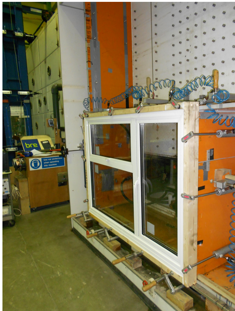
Figure A2. The test specimen installed in the BRE 'G' Weathertightness test rig
