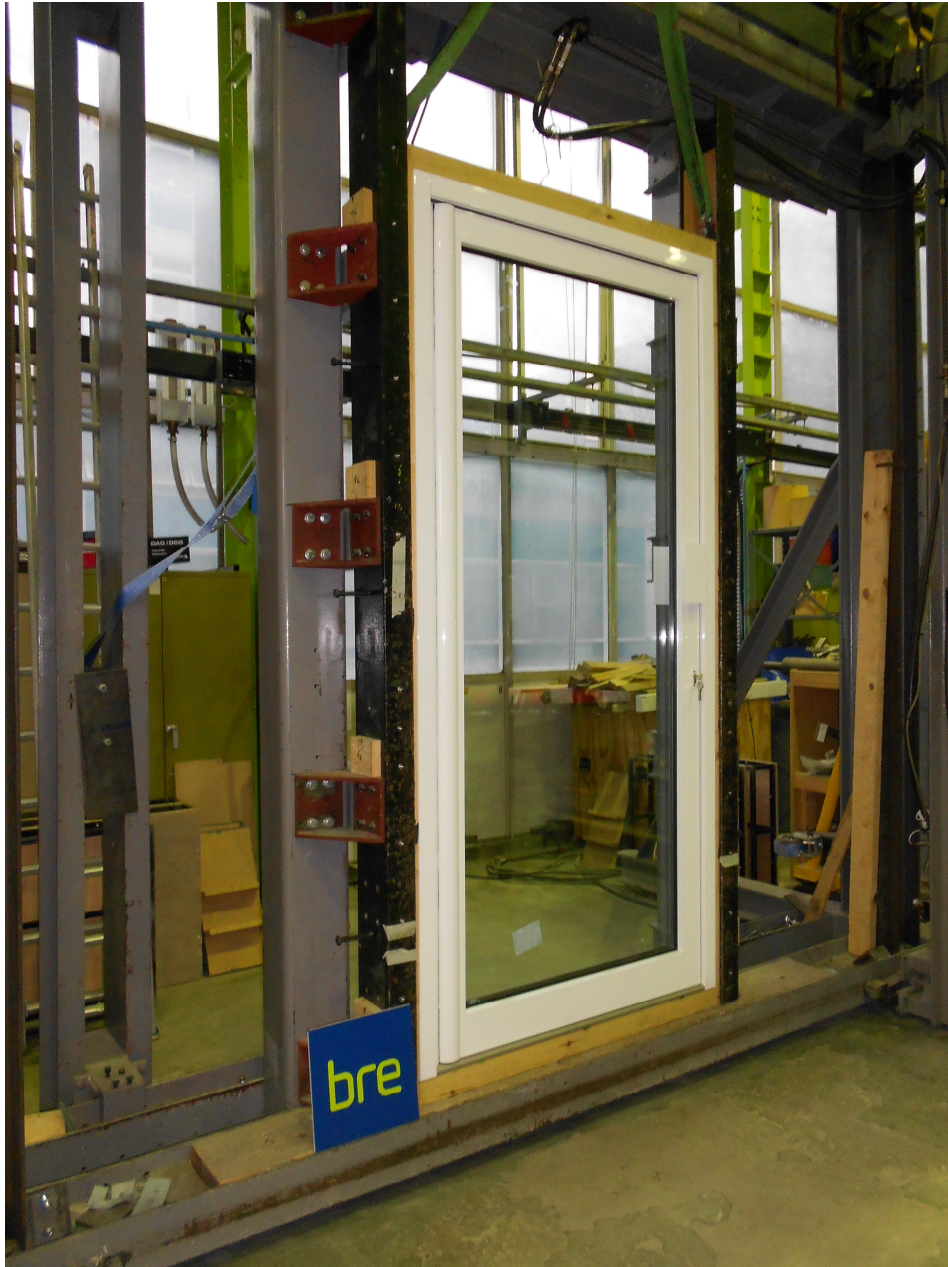
Figure 1. SmartWall single leaf, double swing door installed in the test rig
